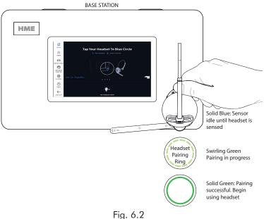
**Notes:** A swirling red light indicates an unsuccessful pairing. Try again by first verifying that the headset is on, and the battery is fully charged. Hold the headset steadily centered and flush against the Headset Pairing Ring (headset movement and distance from the Pairing Ring can cause pairing errors). A weak battery might also result in pairing issues, replace with a fully charged battery as necessary. Registration automatically happens with the initial pairing.
