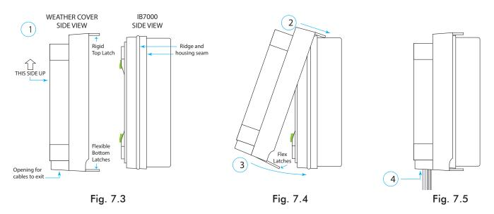
**Note**: To remove the cover, do so in reverse order to the above steps. First, use your fingers to pry the flexible latches on the cover bottom as you detach it from the IB7000 ridge and housing seam it is gripping. Hinge outward away from the IB7000 until the top freely detaches.
